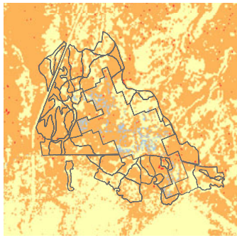
Predicted fire behavior before and after treatments; lighter color indicates a reduced fire severity
