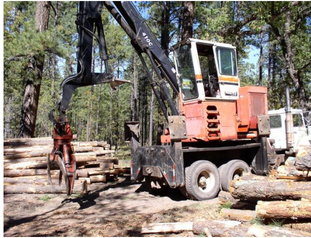
Fig. 5. Harvesting equipment, forest restoration treatment, Apache-Sitgreaves National Forests, AZ.
