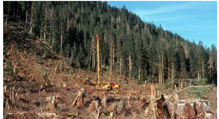
FIG 4. High-lead cable logging like this site on southeastern Chichagof Is. is the dominant methodology used throughout Southeast today, although helicopter logging is also used in a few situations. (John Schoen)
