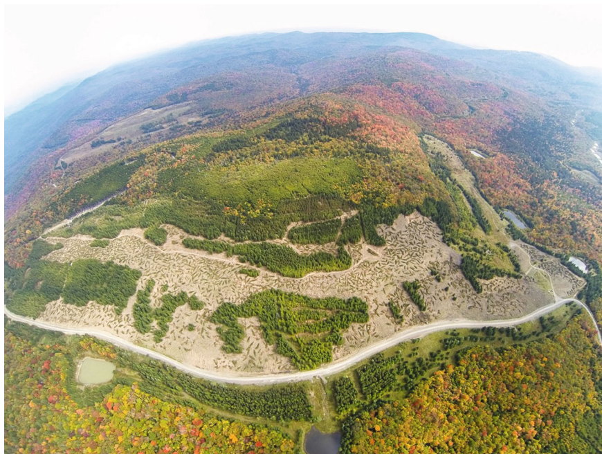
Fig. 9.11 Mower tract mined land restoration site with downed plantations of Norway spruce ( Picea abies ), red pine ( Pinus resinosa ), and other woody debris prior to planting native seedlings and wetland creation (photo by Matt Barton, University of Kentucky Agricultural Communications)
