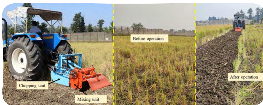
Figure 8: Transition from raw crop stubble (before) to incorporated mulch (after) to prevent residue burning and enhance soil health
