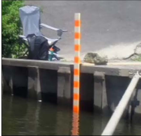
Figure 4: Visual Wake Measurement near a Bulkhead
