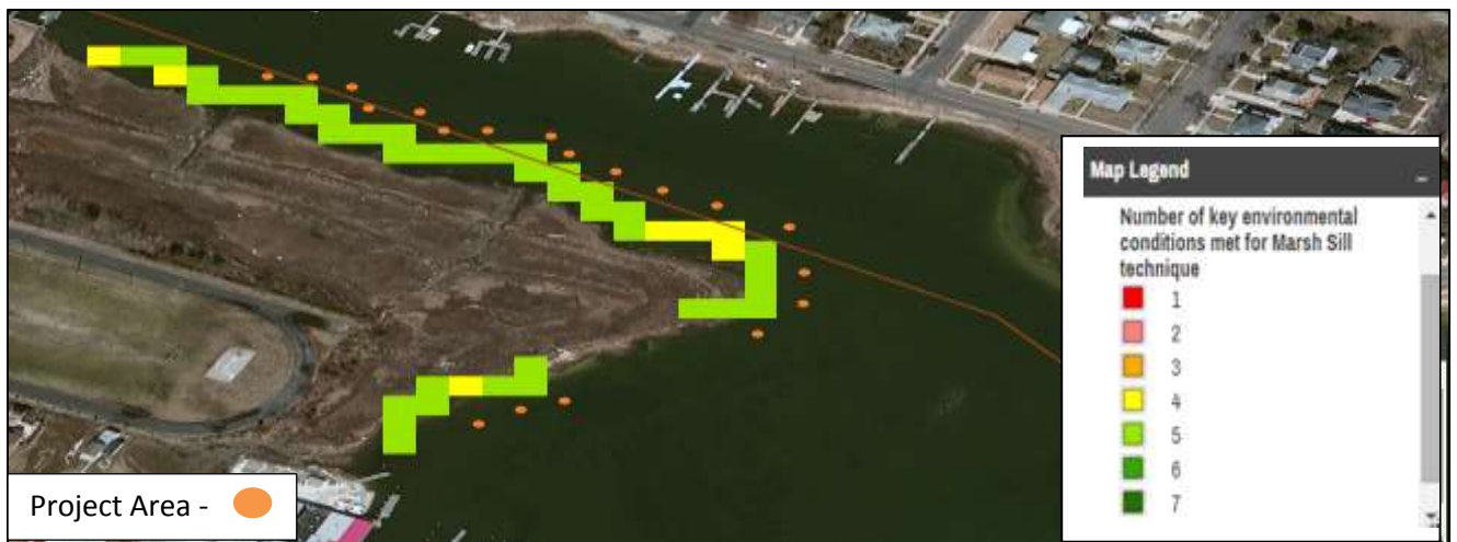
Figure 6. Restoration Explorer information on applicability of a marsh sill at the proposed project location.
