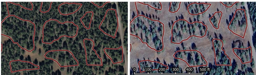
Fig. 2 Digital prescription guides (red lines) on a portion of one treatment unit, overlaid on pre- and post-harvest satellite imagery
