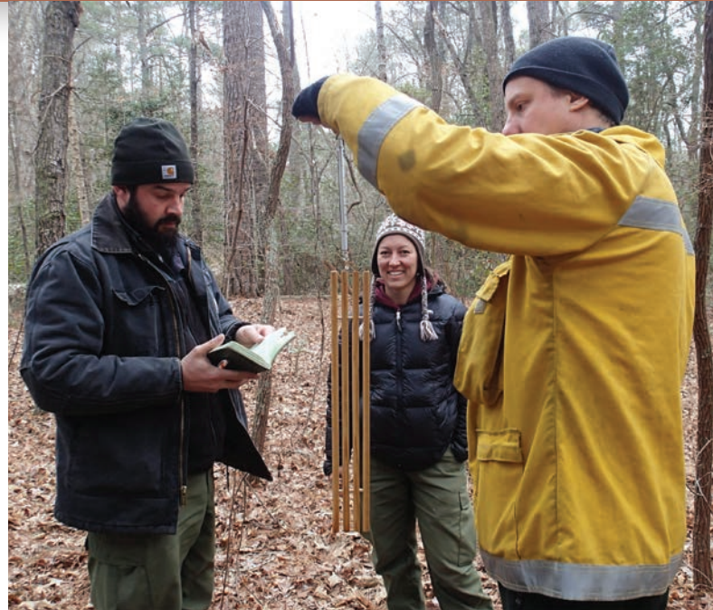
Partners on the Fire Effects Monitoring (FEMO) squad at a Prescribed Fire Training Exchange (TREX) weigh fuel sticks to determine 10-hour fuel moisture. Participants fill roles as trainee and trainer over two weeks of controlled burning and formal training. The HOA FLN has funded dozens of partners to participate across the country. Photo credit: Nikole Simmons TNC
