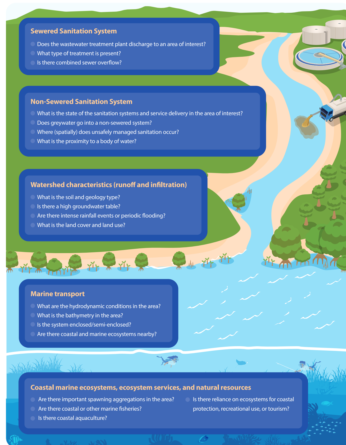
Fig. 6: Factors to consider when assessing whether coastal marine ecosystems and ecosystem services are at risk from wastewater pollution
