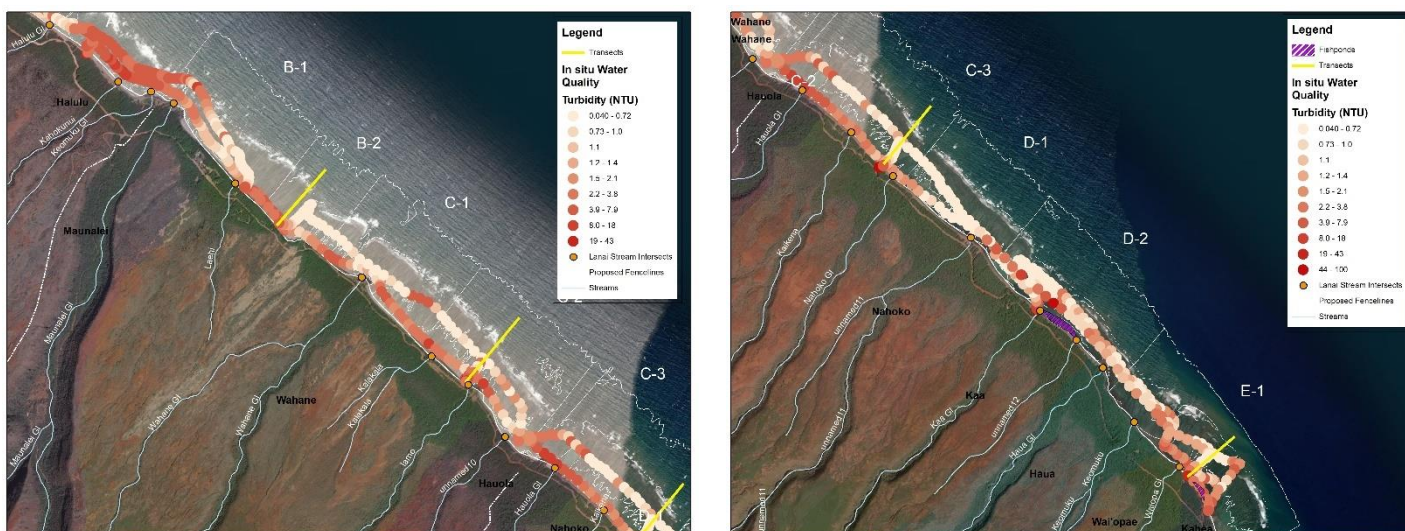
Figure 4.6b. Close-up of turbidity mapping along near (<50m) and far (>250m) transects parallel to shore.
