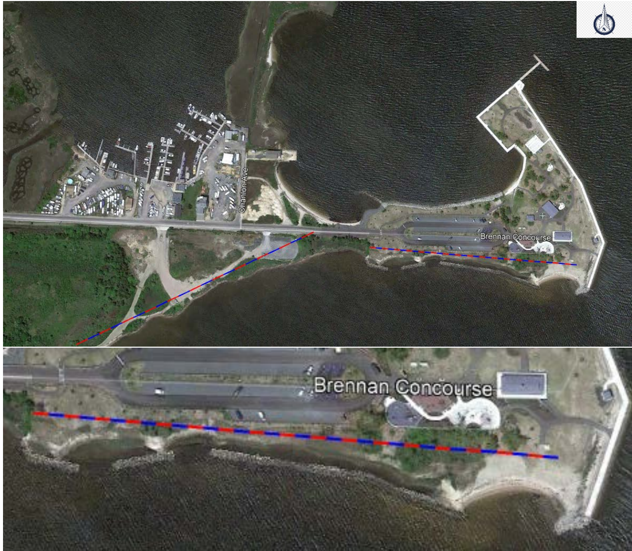
Figure 4: Google Earth Image (May 2019) showing Berkeley Island County Park, Berkeley Township, NJ, at two scales. The red and blue lines on the left in the top image are the baseline for the control area of the shoreline stability analysis. The red and blue line, landward of the breakwater/sill structures, is the baseline for the project area used in the shoreline stability analysis.
