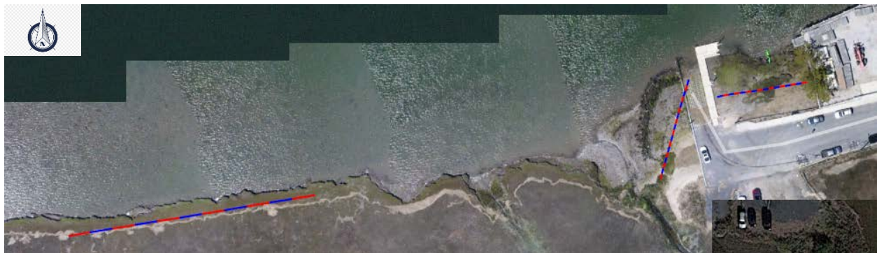
Figure 16: Orthomosaic created from UAV imagery collected on May 7, 2020, showing Strathmere, Upper Township, NJ. The red and blue lines to the left of the image is the baseline for the control area of the shoreline stability analysis. The two red and blue lines, landward of the sill and landward of the vegetated shoreline, to the right of the image are the baselines for the project area used in the shoreline stability analysis.
