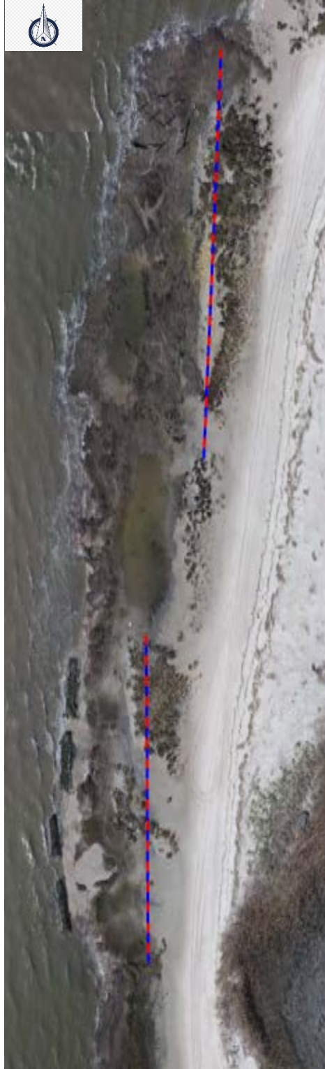
Figure 20: Orthomosaic created from UAV imagery collected on April 6, 2020, showing the Gandys Beach, Downe Township, NJ. The red and blue lines to the North (top) are the baseline for the control area of the shoreline stability analysis. The red and blue line, landward of the Oyster Castle structures at the bottom of the image is the baseline for the project area used in the shoreline stability analysis.
