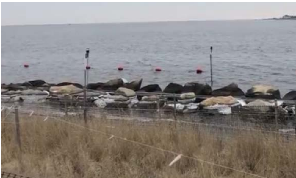
Figure 2: The effectiveness of a sill or breakwater can be evaluated by measuring the waves both in-front-of (offshore) and behind (inshore) the sill or breakwater to calculate effectiveness at attenuating waves under various conditions. Above shows two Wavelogger IIIs deployed at Berkeley Island, NJ, for such purpose in January 2019. The waveloggers are mounted to posts, which are pounded into the ground.
