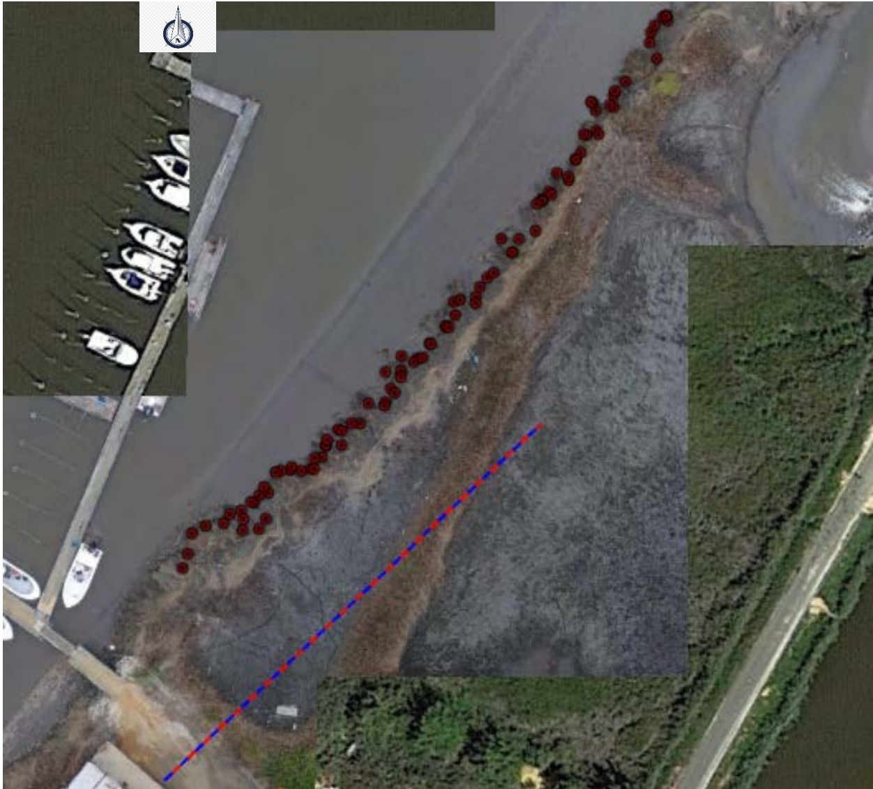
Figure 26: Orthomosaic created from UAV imagery collected on April 7, 2020, showing Matts Landing, Heislerville, NJ. The red and blue line is the baseline for both the control and project area of the shoreline stability analysis. The living shoreline project is along the southern edge of this strip of shoreline, and the control is immediately to the North.
