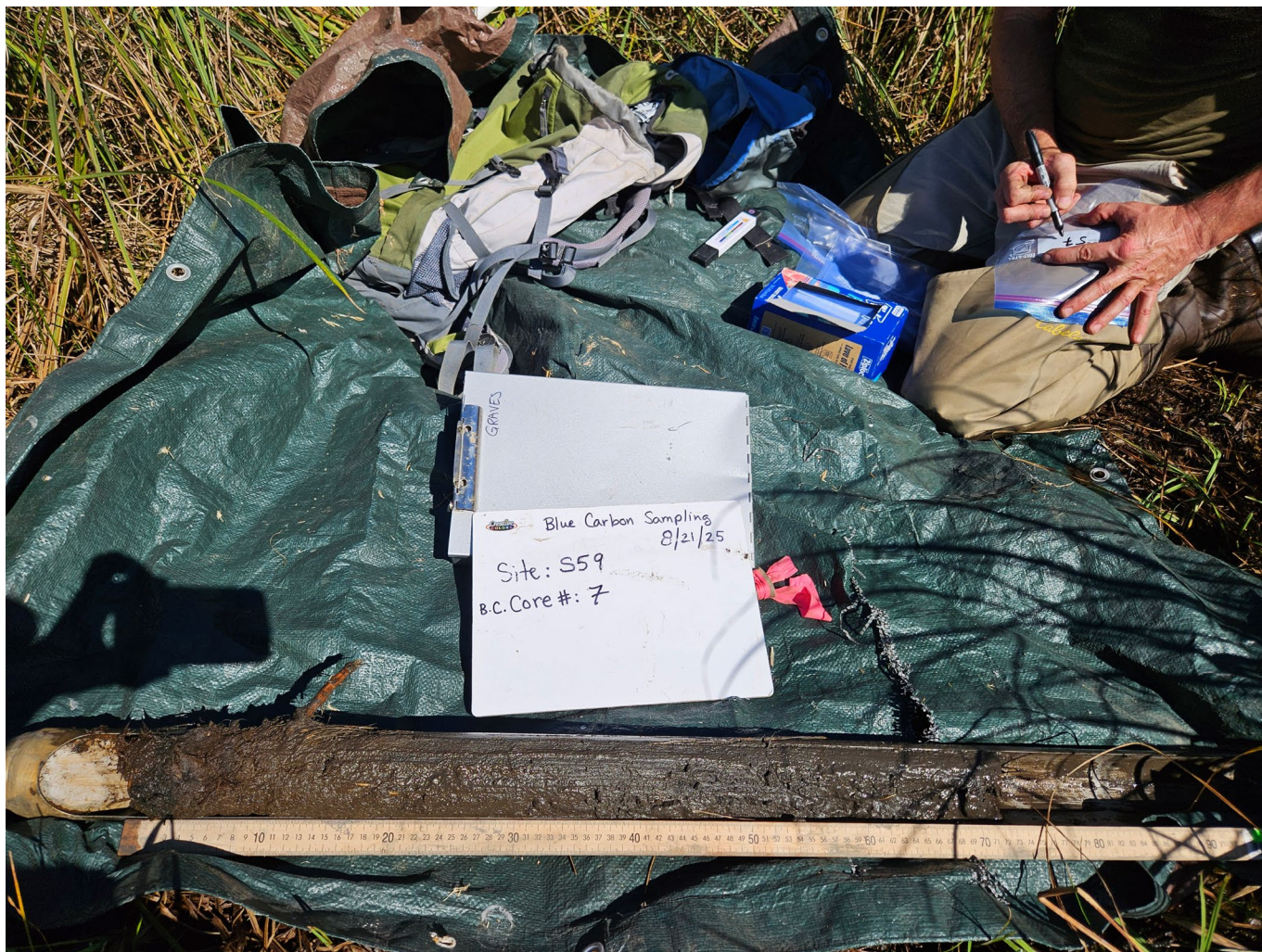
Figure A3. A blue carbon core collected from a tidal marsh in the Siuslaw River Estuary, with gaps that make the core less than fully cylindrical.
