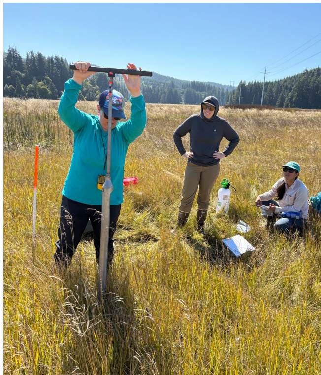
Figure A2. A gouge auger is inserted into a tidal marsh to collect a blue carbon core.
