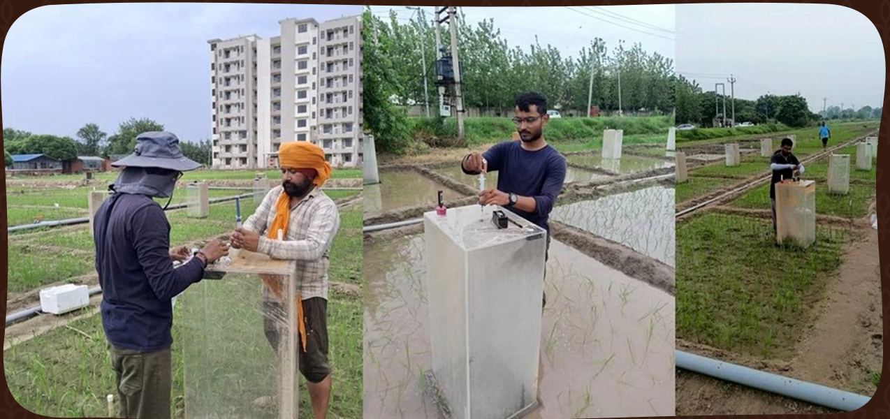
Figure 3: In situ static (closed-cover) flux chamber greenhouse gas sampling process in the experimental plots. Photo credit: IRRRI
