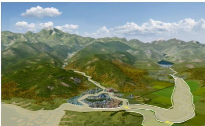
Flood management with green infrastructure during a large flood (e.g., 1 in 100 year frequency). Both bypass and flood detention area are in use. Agricultural land is flooded but primarily land planned to flood; either in flood-compatible crops or with compensation mechanism.
