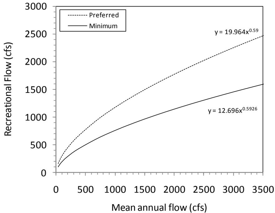
**Figure 15** Recreational flows for canoeing, kayaking and rafting (from Rood et al. 2006). Both the minimum flow and preferred flow are presented (converted to cfs from  $m^3/s$  units of original publication), and Pearson  $R^2$  values for these regression equations were 0.94 and 0.96 respectively.
