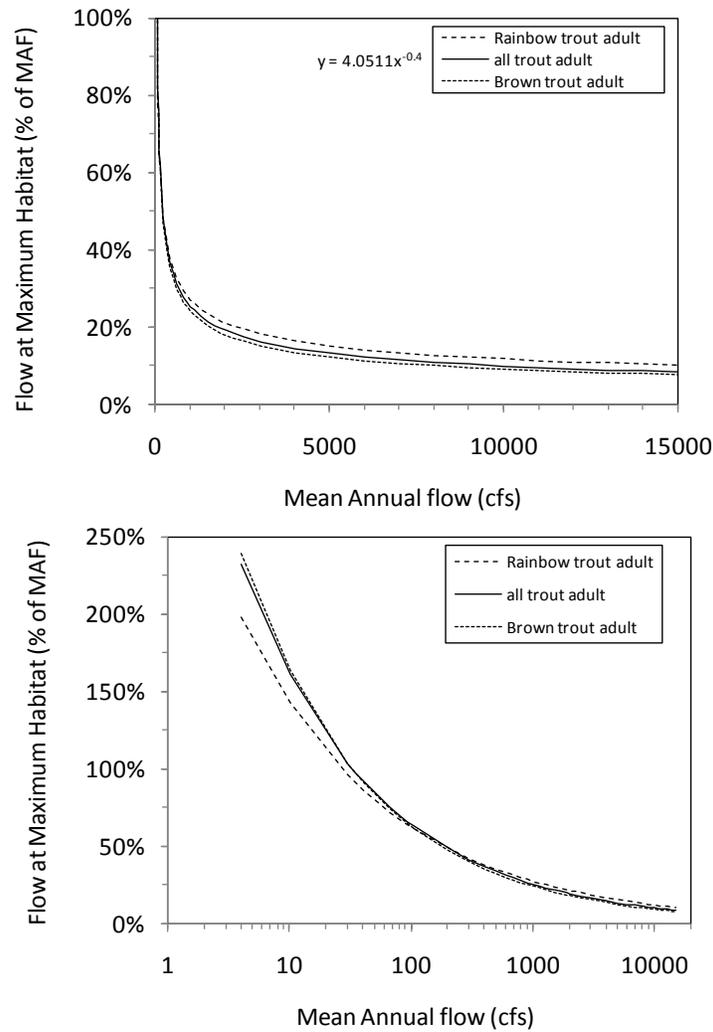
**Figure 11** Relationship of flow for maximum trout habitat to mean annual flow (MAF). The same plot is presented on a linear axis (upper plot) and log axis (lower plot) for mean annual flow. Equations were derived from Hatfield and Bruce (2000) for a scenario of latitude  $41^\circ$  (latitude is a second factor in the models for rainbow trout and “all trout”). The equation for “all trout” is presented (see upper-graph), after conversion from  $m^3/s$  to cfs.
