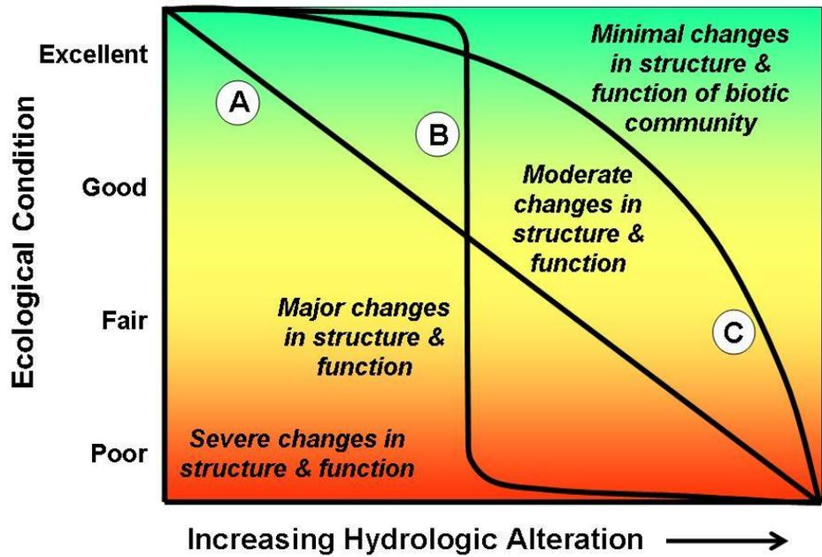
**Figure 2** Three of several possible forms of flow alteration-ecological response relationships: linear (A), threshold (B), and curvilinear (C). The form of the curve depends on the specific ecological and hydrological variables analyzed. (Adapted from Davies and Jackson 2006).
