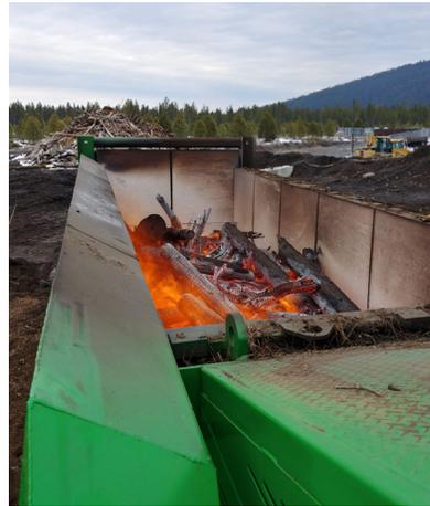
The unit pictured has been used to burn somewhere between 60 and 100 yards of material per day; this varies with the kind of material being loaded, and may increase with more experience. The ash produced is minimal. Nine days of burning yielded about a cubic yard of ash.
