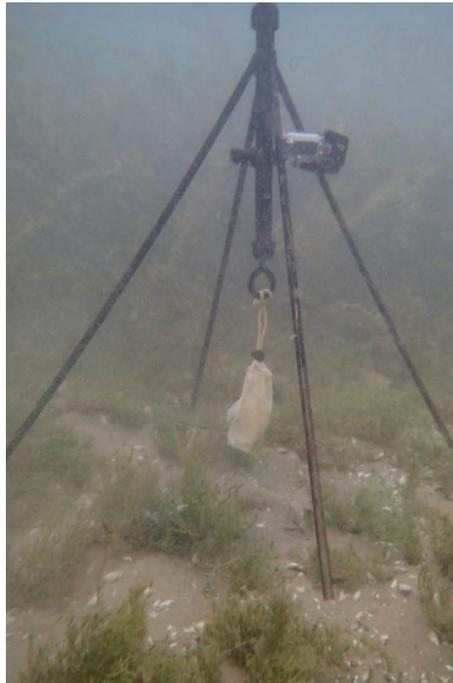
Figure 3.1. The steel rod photoquadrat frame used in Lake Michigan to assess benthic fish abundance. Each quad-pod frame was baited with Lake Trout (*Salvelinus namaycush*) eggs and had a downward facing GoPro<sup>®</sup> camera attached to the center.
