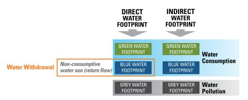
Figure 2. Components of a Water Footprint Source: Water Footprint Manual (2009)
