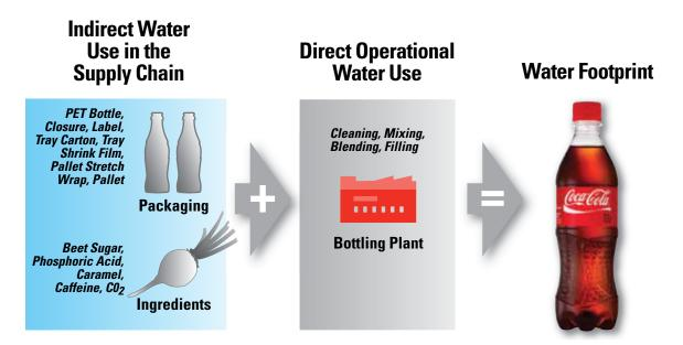
**Figure 4. Indirect and Direct Water Footprint Components**
