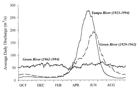
**Figure 1** Typical flows over a water-year (average daily flow, October-September) comparing three sites. The dashed line represents flows for Green River before Flaming Gorge Dam was built – compare that to the post-dam flows for 1962-1994. This graph also shows flows for the unregulated Yampa River. Graph from Merritt and Cooper 2000.
