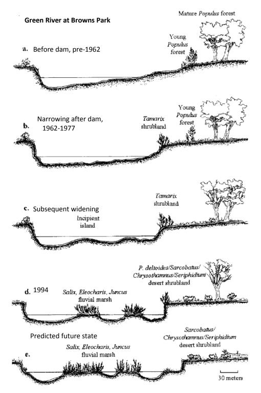
**Figure 2** Changes in channel and vegetation in the Green River at Browns Park, showing typical cross-section before and after construction of Flaming Gorge Dam. From Merritt and Cooper (2000).
