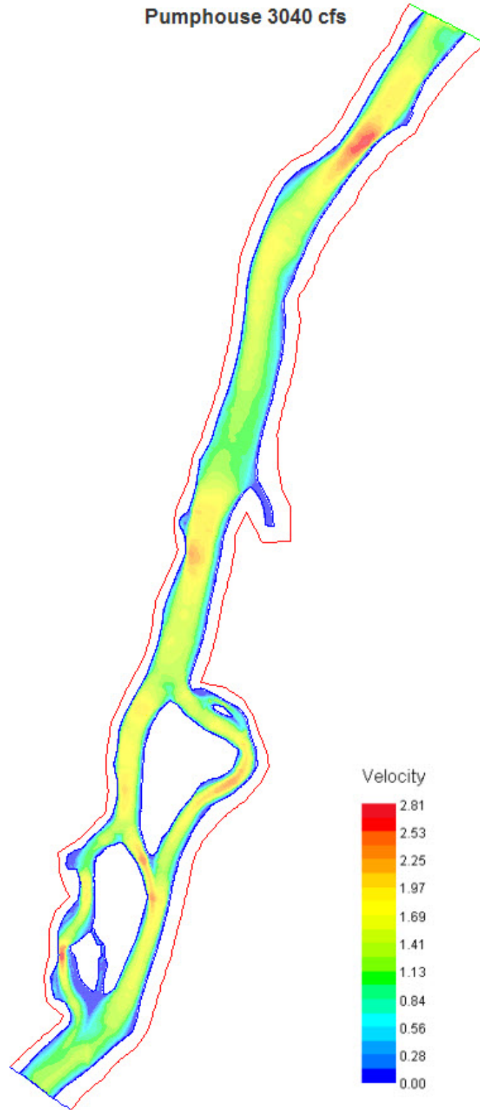
Figure 33. Pumphouse simulated water velocity (m/s) at 3040 cfs (high flow). Flow moves from top to bottom.
