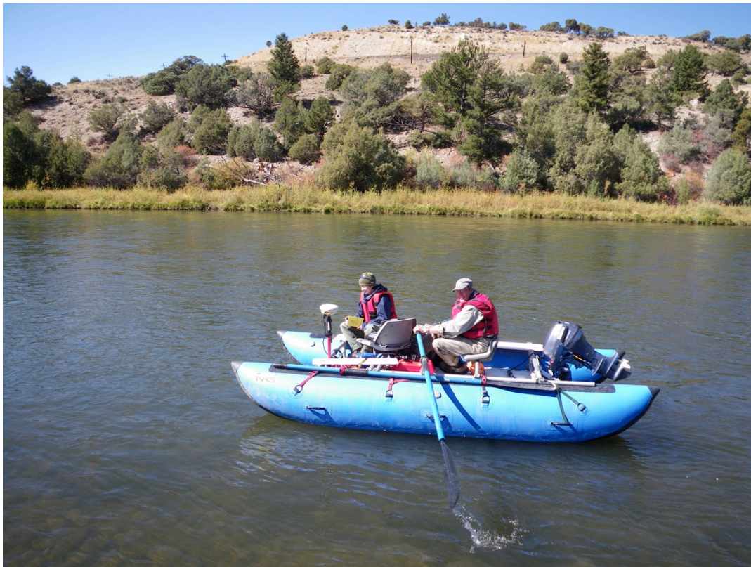
Figure 14. Floating a longitudinal transect at Pumphouse to collect streambed elevation, velocity, and depth information.
