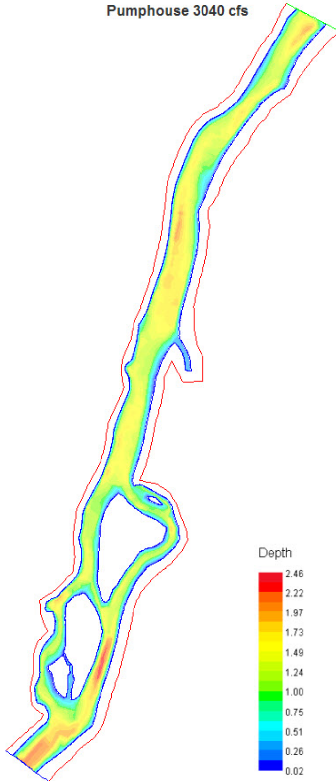
Figure 34. Pumphouse simulated water depth (m) at 3040 cfs (high flow). Flow moves from top to bottom.
