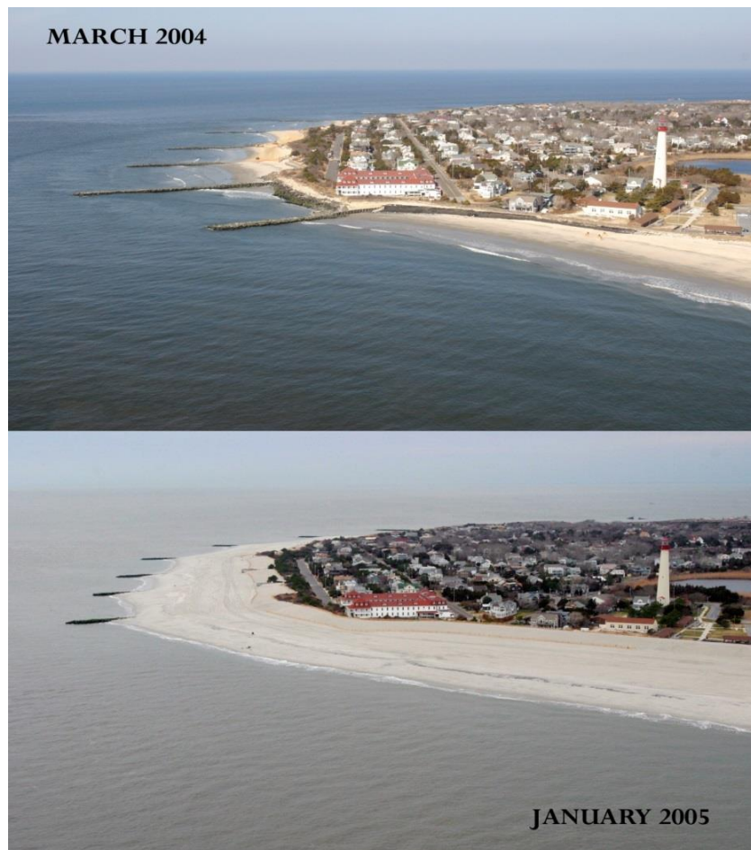
Figure 2. Beach replenishment on the state park beach and around Cape May Point, before and after the restoration Source: U.S. Army Corps of Engineers 2007
