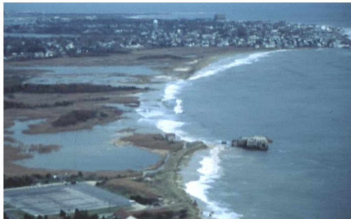
Figure 2. Lower Cape May Meadows during the dune breach in the October 1991 storm Source: U.S. Army Corps of Engineers (1991)
