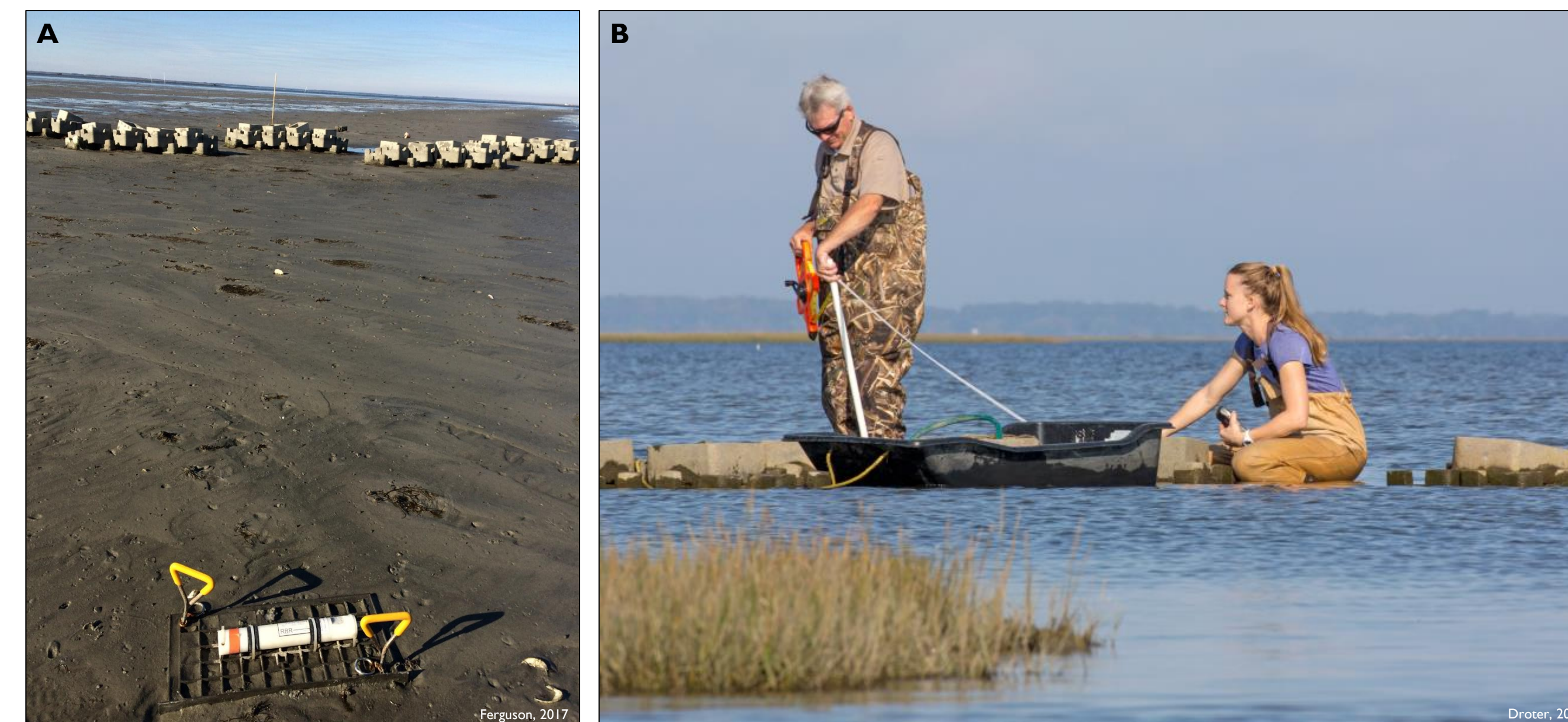
Figure 3. Wave gauges were placed along a transect on either side of the reef at Chincoteague Reef (A, B). The sensors measure changes in pressure to determine water depth; water depth fluctuations about the mean water level are used to resolve wave height.
