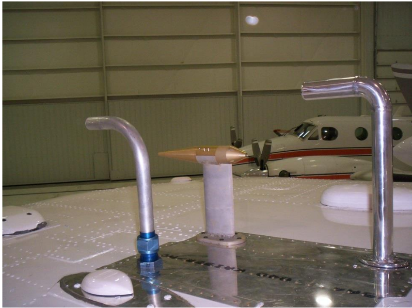
Inlets on Twin Otter roof
