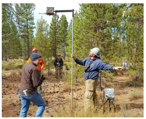
Mark Stern assisted the team of scientists from the University of Montana W.A. Franke College of Forestry & Conservation in installing instruments to collect data on thermal flux, temperature and rate of fire spread. GoPro cameras also took video of fire conditions. In addition to the instruments installed on the pole, similar instruments were placed the boxes (seen here, wrapped in what looks like aluminum foil) and 38 anemometers measured wind speed and direction in and around the burn areas.
