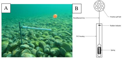
Figure 3. A) Picture of maximum wave velocity dynamometer deployed at the reference site.
