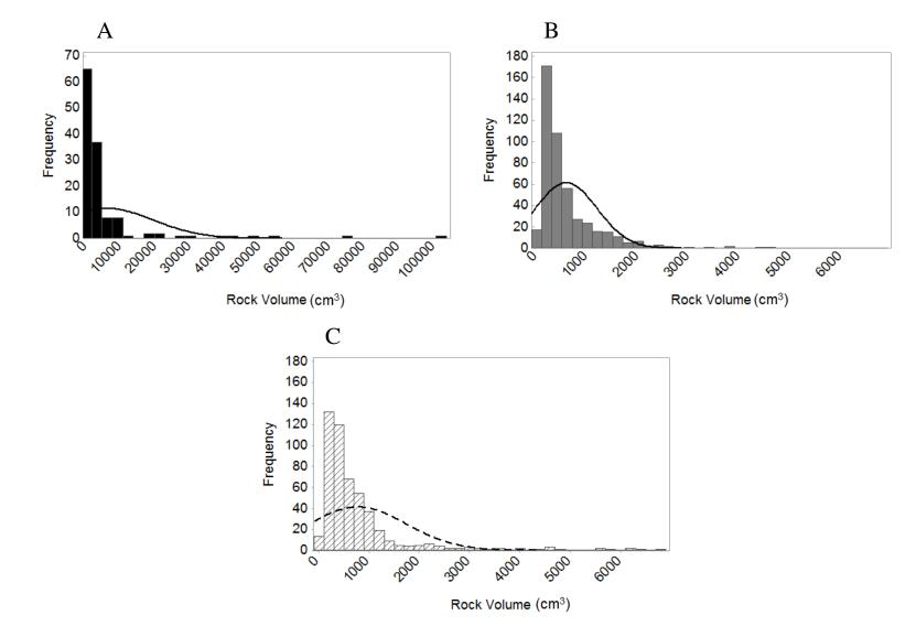
Figure 4. Occurrence frequency of the pre-restoration (A), reference (B), and post-restoration (C) individual rock volumes. Individual rock volumes were calculated by taking the product of the x, y, and z axes measurements from each rock.
