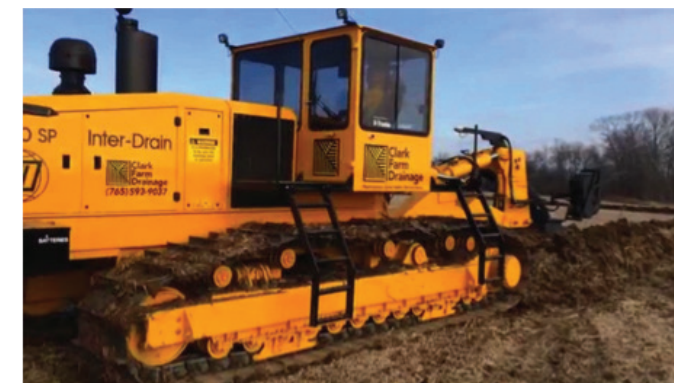
Installing a 12" main with an Inter-Drain 2050 SP. Photo courtesy of Clark Farm Drainage.
