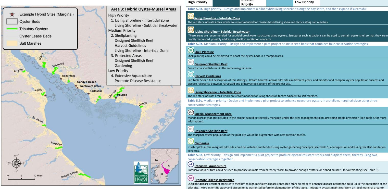
Figure 5.33. Area 3: Locations of potential hybrid tactic areas incoporating living shorelines, oyster breakwaters, and tributary oyster beds
