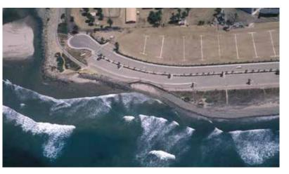
**Before project construction:** Coastal erosion had destroyed a bike path and damaged a parking area for the Ventura County Fairgrounds.
