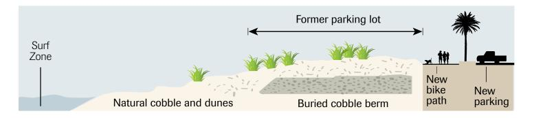
Under the managed retreat plan, the bike path and parking lot were relocated inland (below). An eight-foot-thick berm of cobblestones beneath vegetated dunes was built in place of the parking lot (above), restoring habitat and beach processes while providing erosion protection.
