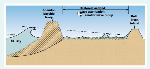
**Figure 1:** Tidal marshlands reduce wave energy substantially. Modeling results indicate that it would be cost-effective to abandon deteriorating bayshore levees in favor of smaller levees built landward of restored tidal marshes. This strategy would meet both ecological restoration and long-term flood risk management goals.
