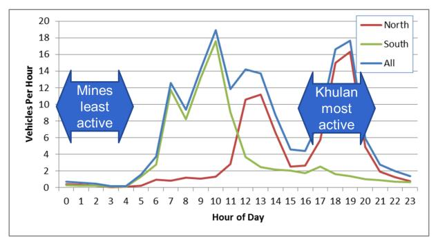
Figure 21: Existing Traffic on OT-GS Road with Potential Times for Traffic Restrictions
