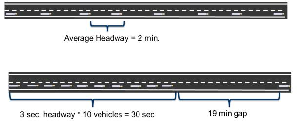
Figure 25: Conceptual Example of Truck Platooning (not to scale)
