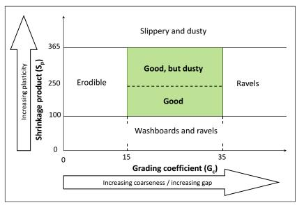
Figure 27: Material performance predictor chart (adapted from Paige-Green, 1989)
