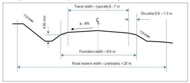
An example cross-section of an unpaved road is shown in Figure 29.
