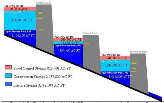
Figure 3. Profile schematic of the USACE reservoir system on the Savannah River
