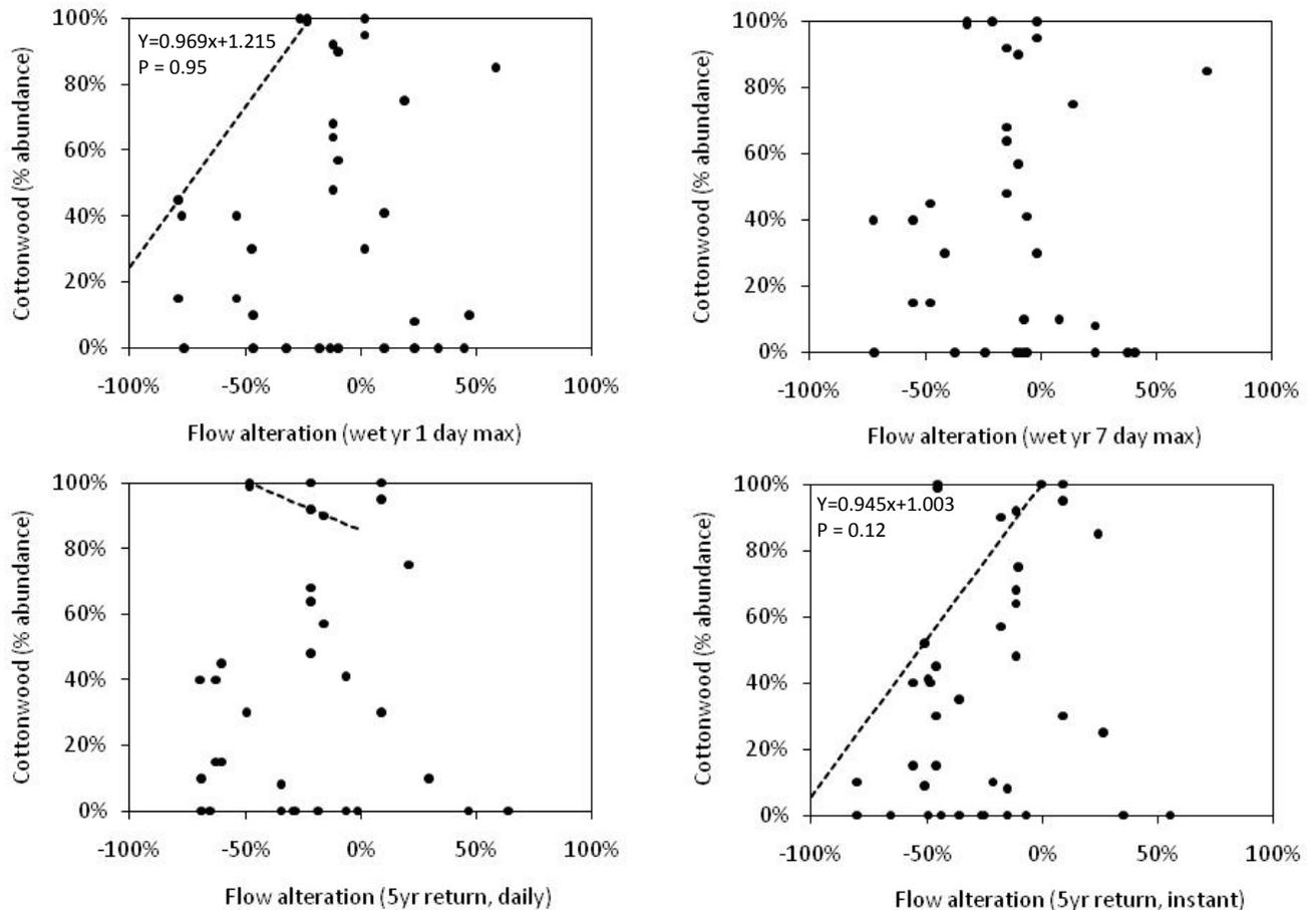
**Figure 5.** Adult cottonwood response to peak flow alteration. This plot includes two “wet year” average maxima (1-day and moving 7-day average), the daily series 5-year return period maxima and instantaneous 5-year return maxima. The dashed lines are 90% quantiles fit to the data ( $y=100\%$  for 7-day).
