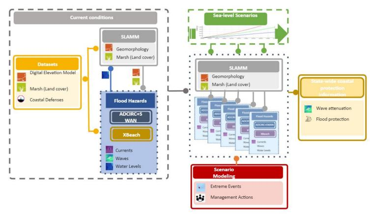
*Figure 2.* Depiction of the modeling framework being used to estimate the wave attenuation capacity of natural and nature-based features across Maryland.
