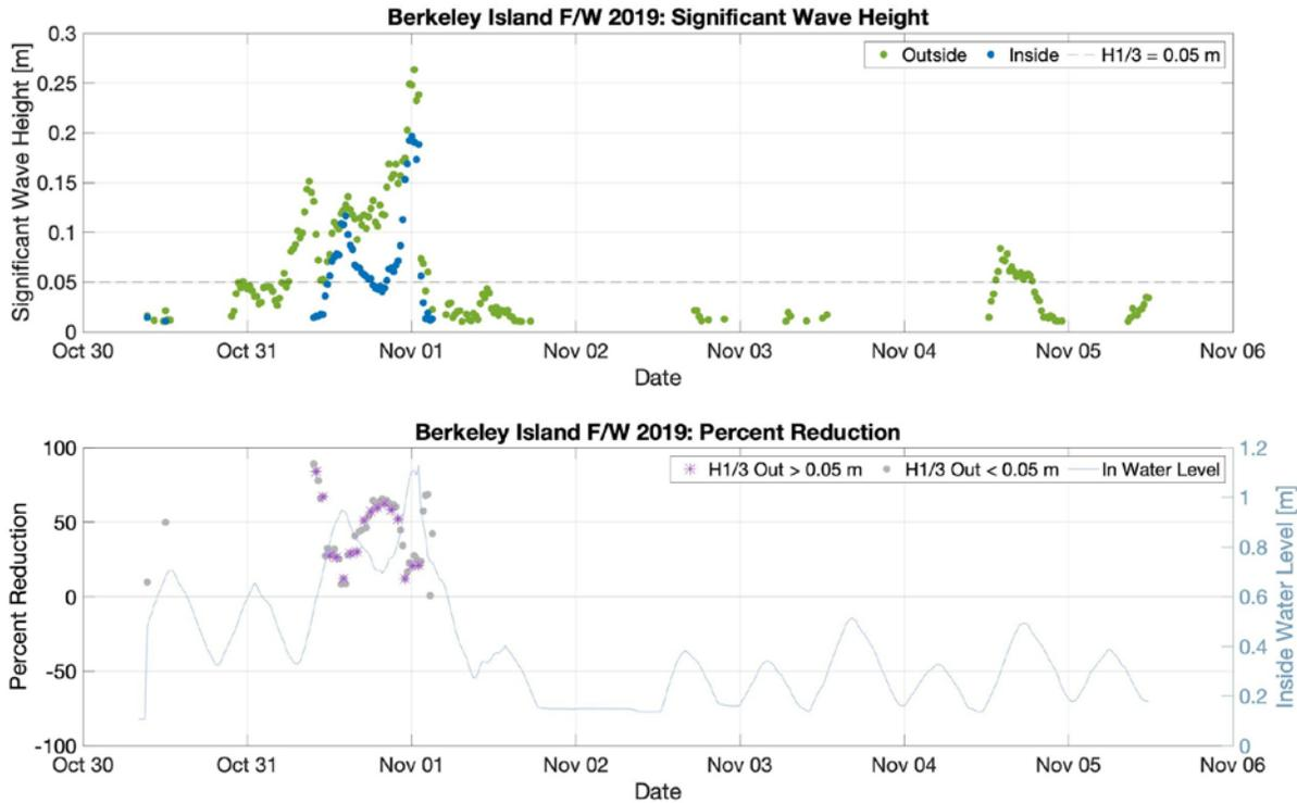
*Figure 7: Significant wave heights, percent reduction and inshore water level for Berkeley Island during the fall/winter 2019 monitoring period. All percent reduction values are shown in gray, and purple stars were added to highlight periods when offshore significant wave heights exceeded 5 cm.*
