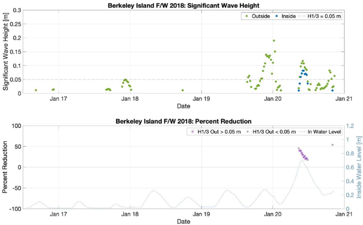
Figure 34: Significant wave height and percent reduction for Berkeley Island fall/winter 2018 deployment.
