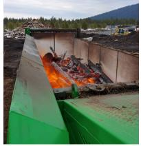
The unit pictured has been used to burn somewhere between 60 and 100 yards of material per day; this varies with the kind of material being loaded, and may increase with more experience. The ash produced is minimal. Nine days of burning yielded about a cubic yard of ash.
