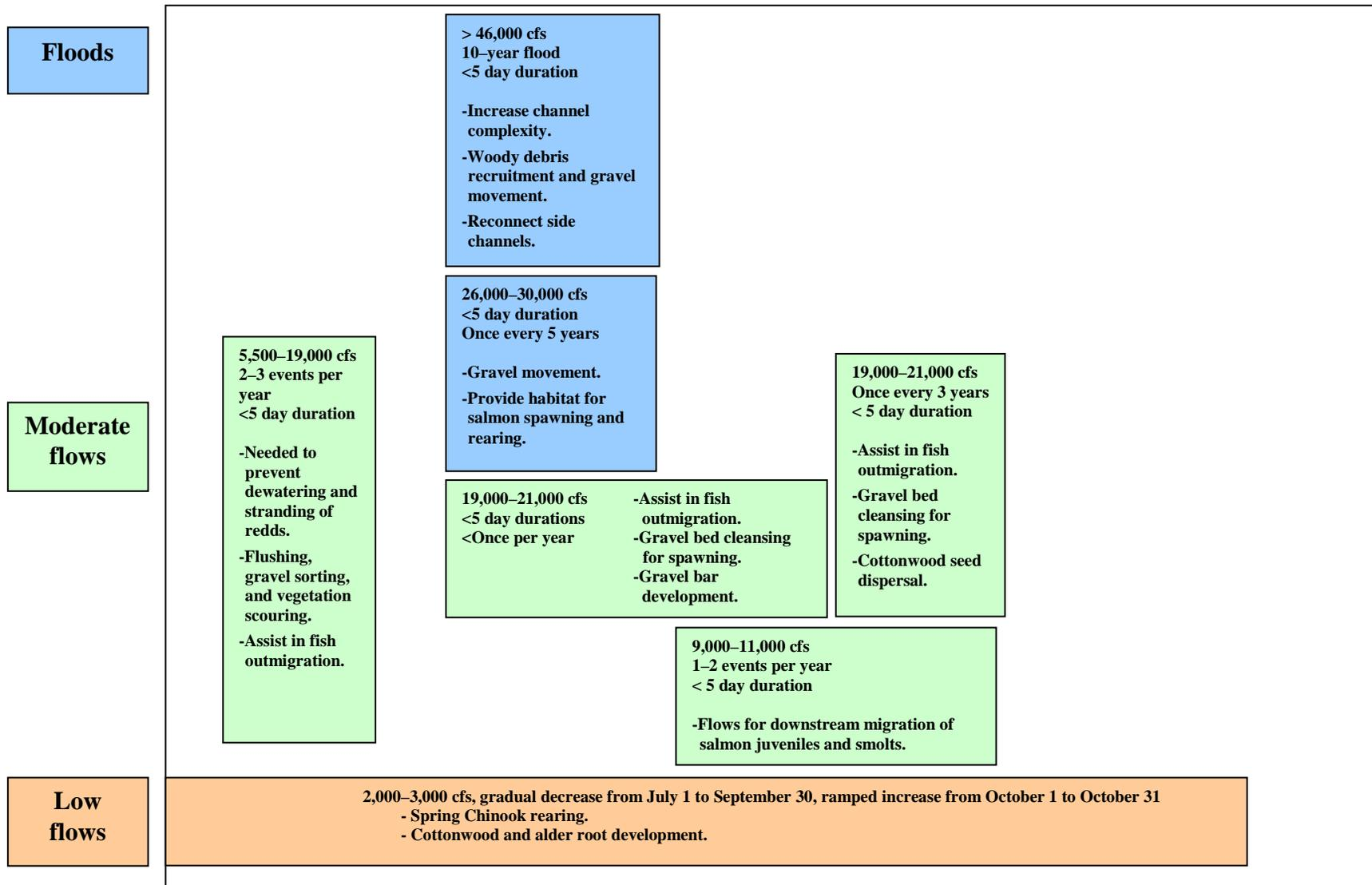
Figure 5. Dam flow release and ecology linkages for the Middle McKenzie River (Reaches 4–7)
