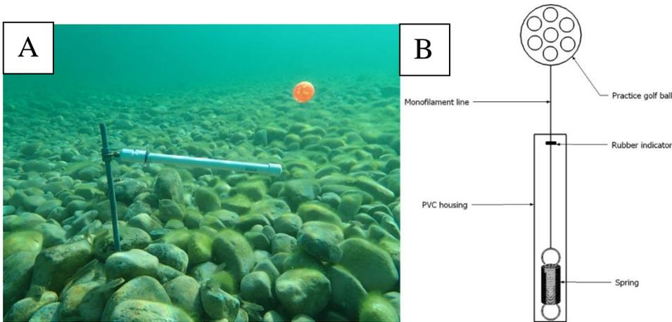
435 Figure 3. A) Picture of maximum wave velocity dynamometer deployed at the reference site.
