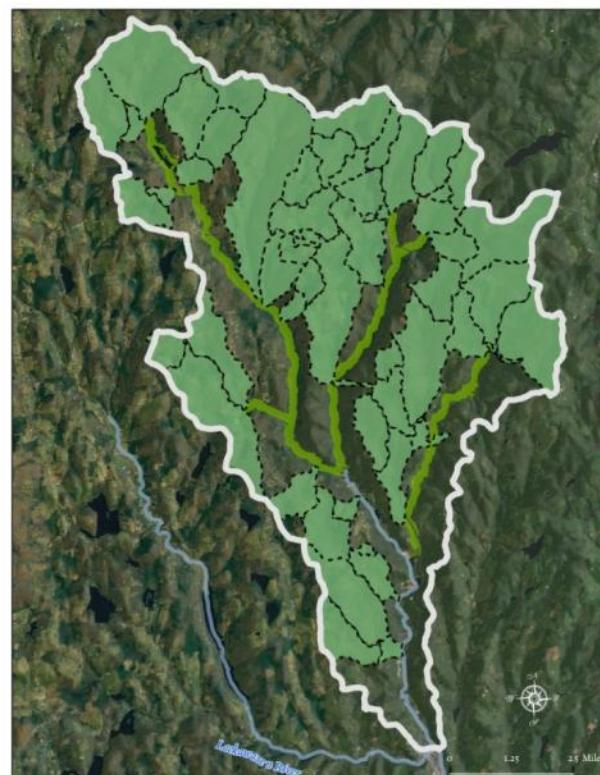
**Figure 3. Headwater Network for the Dyberry Creek . Headwater networks are defined by small catchments (<3.861 mi<sup>2</sup>) linked to downstream riparian corridors and summed to the HUC10 watershed.**
