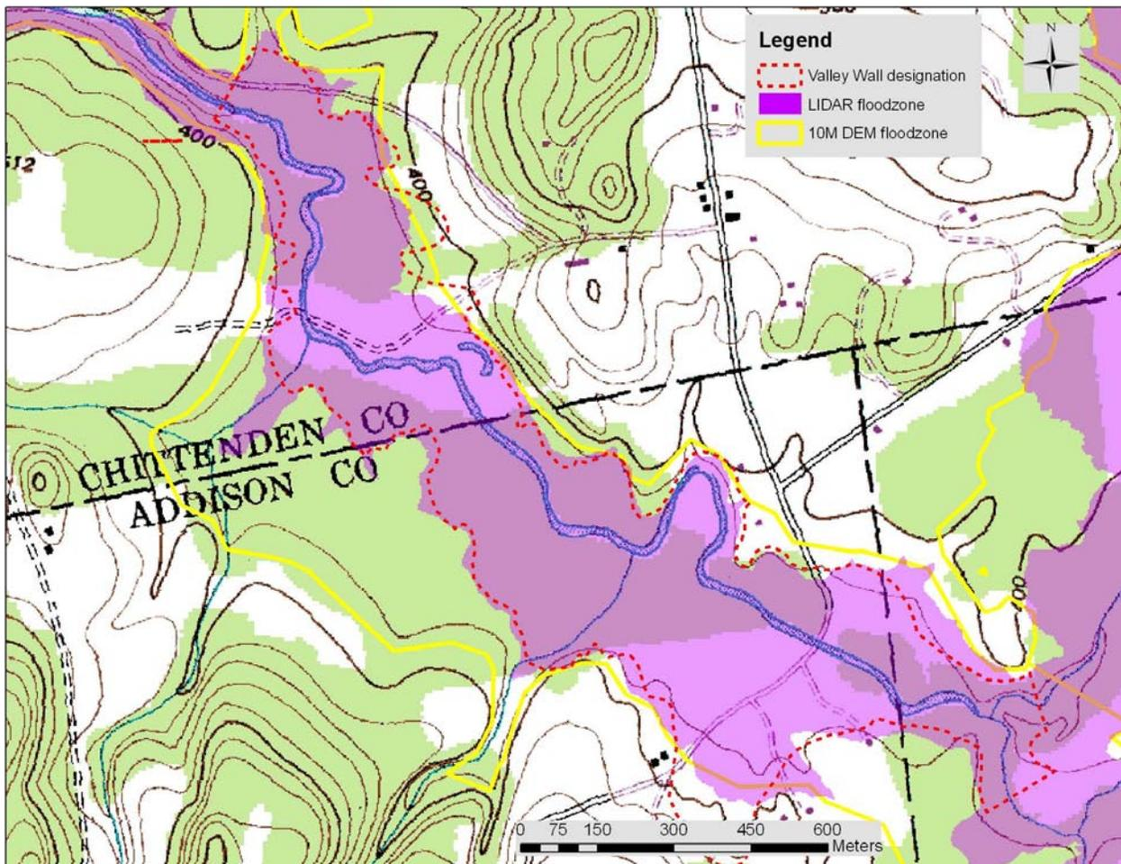
Figure 4: Comparison of LIDAR derived floodzone, 10m DEM floodzone, and VTDEC RMP valley wall designation on reach M15. Note that the LIDAR derived floodzone closely corresponds to the RMP valley wall designation.
