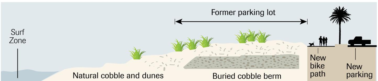
Under the managed retreat plan, the bike path and parking lot were relocated inland (below). An eight-foot-thick berm of cobblestones beneath vegetated dunes was built in place of the parking lot (above), restoring habitat and beach processes while providing erosion protection.
