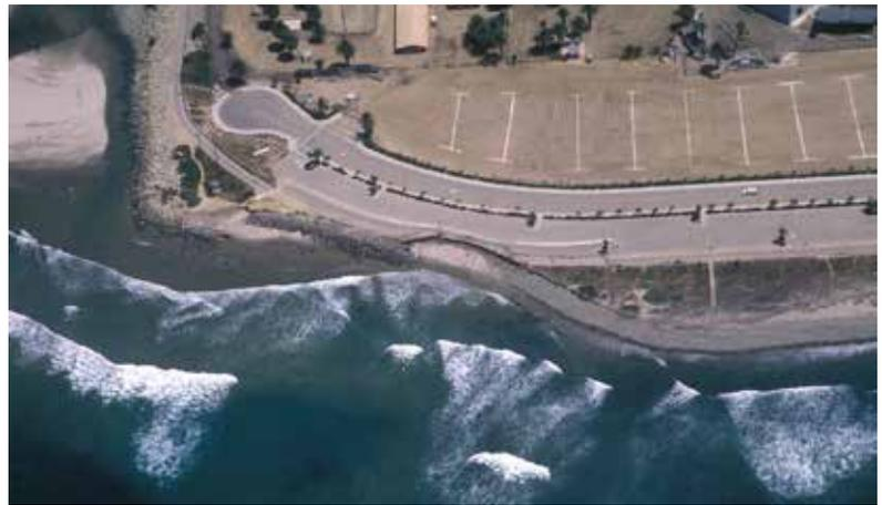
**Before project construction:** Coastal erosion had destroyed a bike path and damaged a parking area for the Ventura County Fairgrounds.
